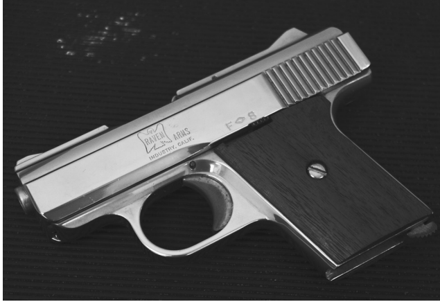
Figure 4.1 (See color insert.) The Raven MP-25. Part of the identification markings are on left side of the slide (pictured); the model and caliber are on the opposite side. The serial number is stamped on the back strap of the grip. The Raven pistols are grouped as one of the Saturday night specials; untold millions were made, and they routinely turn up. (Image from author's collection.)
